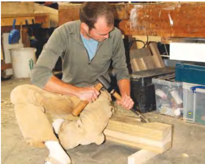
▲ Pic.9 The standard Japanese position for chiselling. The wall-plate is raised up on blocks
